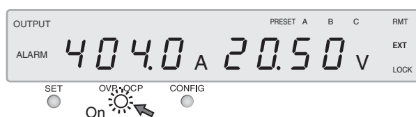
Fig.4-3 Setting display example of the overvoltage and overcurrent protection
