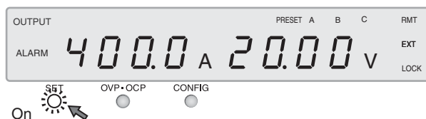
Fig.4-2 Setting display example of the output voltage and output current
